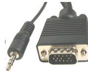
CONNECT VGA CABLE (Macs require an adapter) Audio cable to computer headphone jack if required
